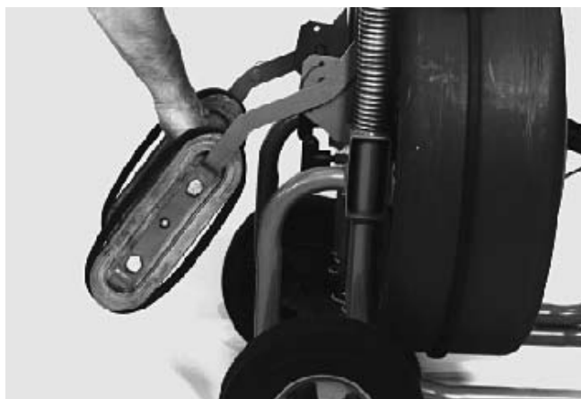
Figure 3 – Relevage du monte-marches
