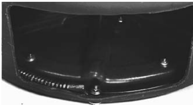
Figure 24 – Anchoring of Pigtail in Drum
