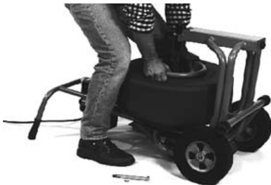
Figure 20 – Lifting Drum Assembly Onto Frame
