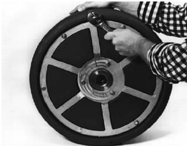
Figure 23 – Removing Pigtail Anchoring Bolt
