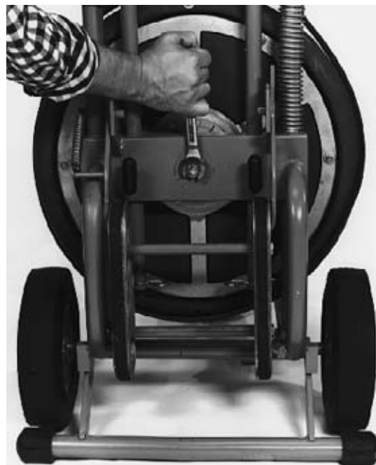
Figure 19 – Removing Rear Support Bolt
